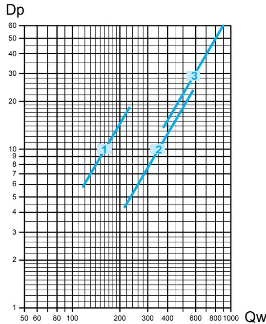
Pressure drop for mean water temperature of 65°C; for different temperatures multiply the pressure drop figure by the K correction factors in the table.
