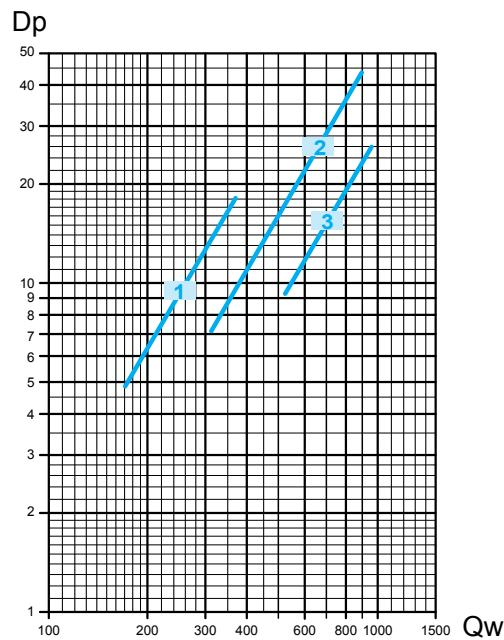
Pressure drop for mean water temperature of 10°C; for different temperatures multiply the pressure drop figure by the K correction factors in the table.
